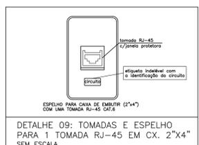
DETALHE 09: TOMADAS E ESPELHO PARA 1 TOMADA RJ-45 EM CX. 2"x4" SEM ESCALA
